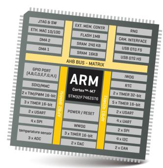
Figure 2: STM32F746ZGT6 MCU block schematic
