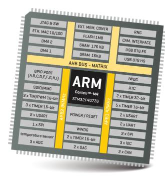
Figure 1: STM32F407ZGT6 MCU block schematic
